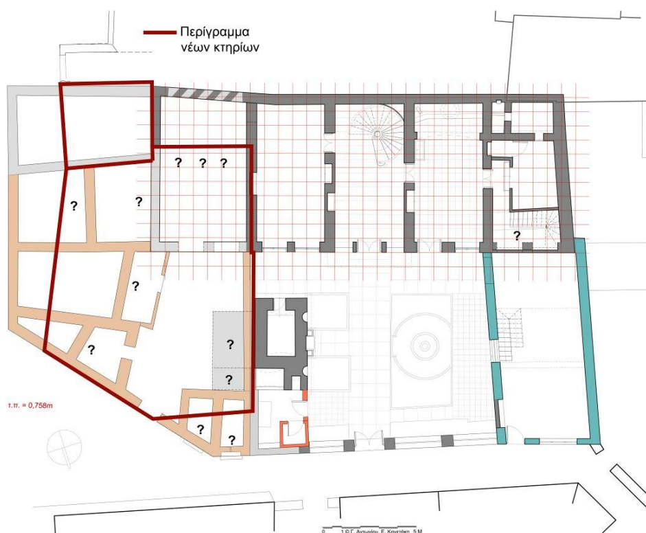
Fig.5: Ground floor plan indicating the constructional phases. (The modern building is indicated with a red outline). Source: G. Antoniou, 2016
